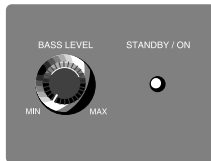
Figure 4: Front Panel Variable Level Control located behind the removable grille.
