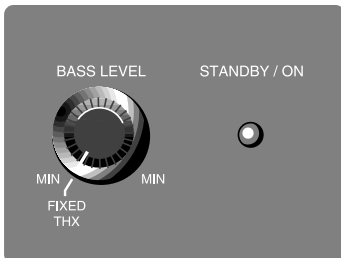
Figure 5: Front Panel Variable Level Control located behind the removable grille
