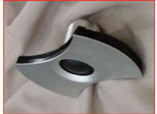
More than meets the eye: Atlantic's LRT has a special rear chamber that lets the tweeter respond lower, and it also functions as a large heat sink, for great power handling.
