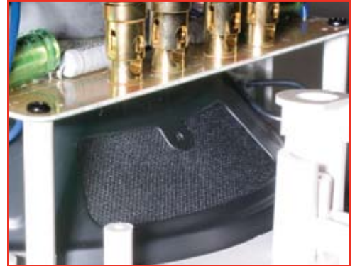
Figure 1 Debris shield prevents contamination
