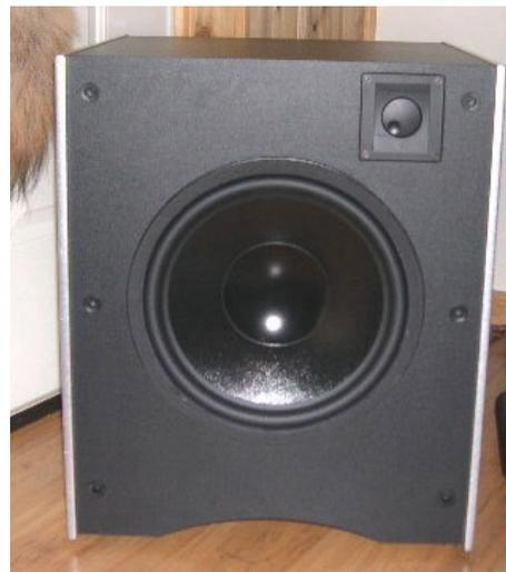
The Atlantic Technology design studio worked hard on the aesthetic presentation to ensure this subwoofer was more than just a "big black box", and I think they succeeded. The sides of the subwoofer feature a subtle horizontal convex geometry, with shaved top edges and arches at the bottom. The top, rear, and bottom surfaces are flat black, and the sides are painted in a silver metallic finish.
